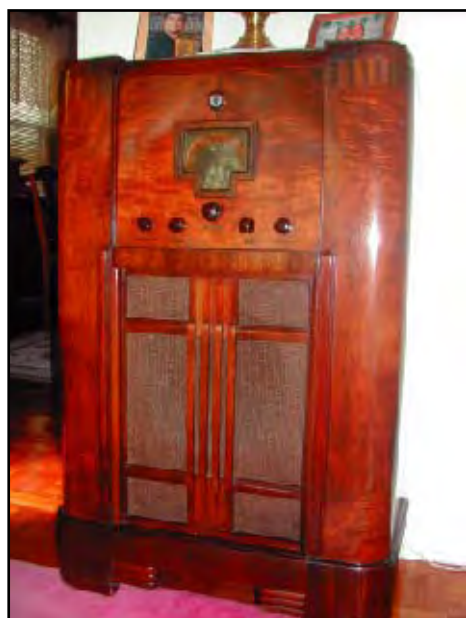
RCA VICTOR Shortwave and AM tube radio. Featured a Light called the Magic Eye,(seen at very top) that lit up when a station got tuned in and on frequency.
