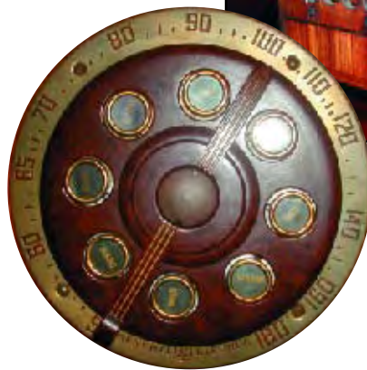
General Electric AM tube radio with a push button dial that rotated for desired station WABC, WOR etc...
